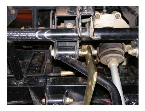
Note location of washer between bracket and factory frame below
