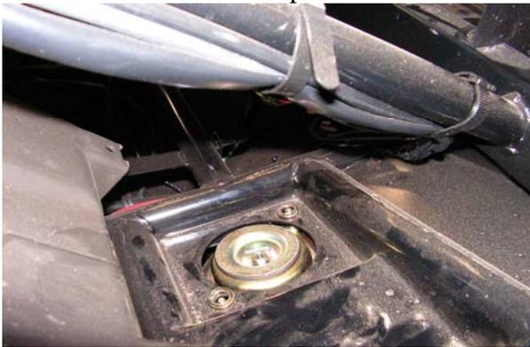
5.) Leaning the strut forward toward the headlamp buckets will put the strut in position to allow you to reach over the top and place the strut spacer in place. Install the strut spacer on top of the coil retainer and tightening the nuts. Install the supplied gasket on top of the strut spacer, and re-install the strut assembly.
