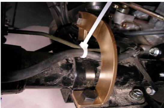
4.)Make sure none of the hoses or brake lines are pinched or in a bind, then reinstall tires and lower to the ground.
