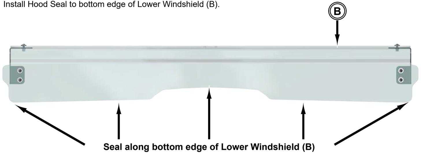
*To ease installation, soak Seal in hot water before cutting or installing to increase flexibility.*
