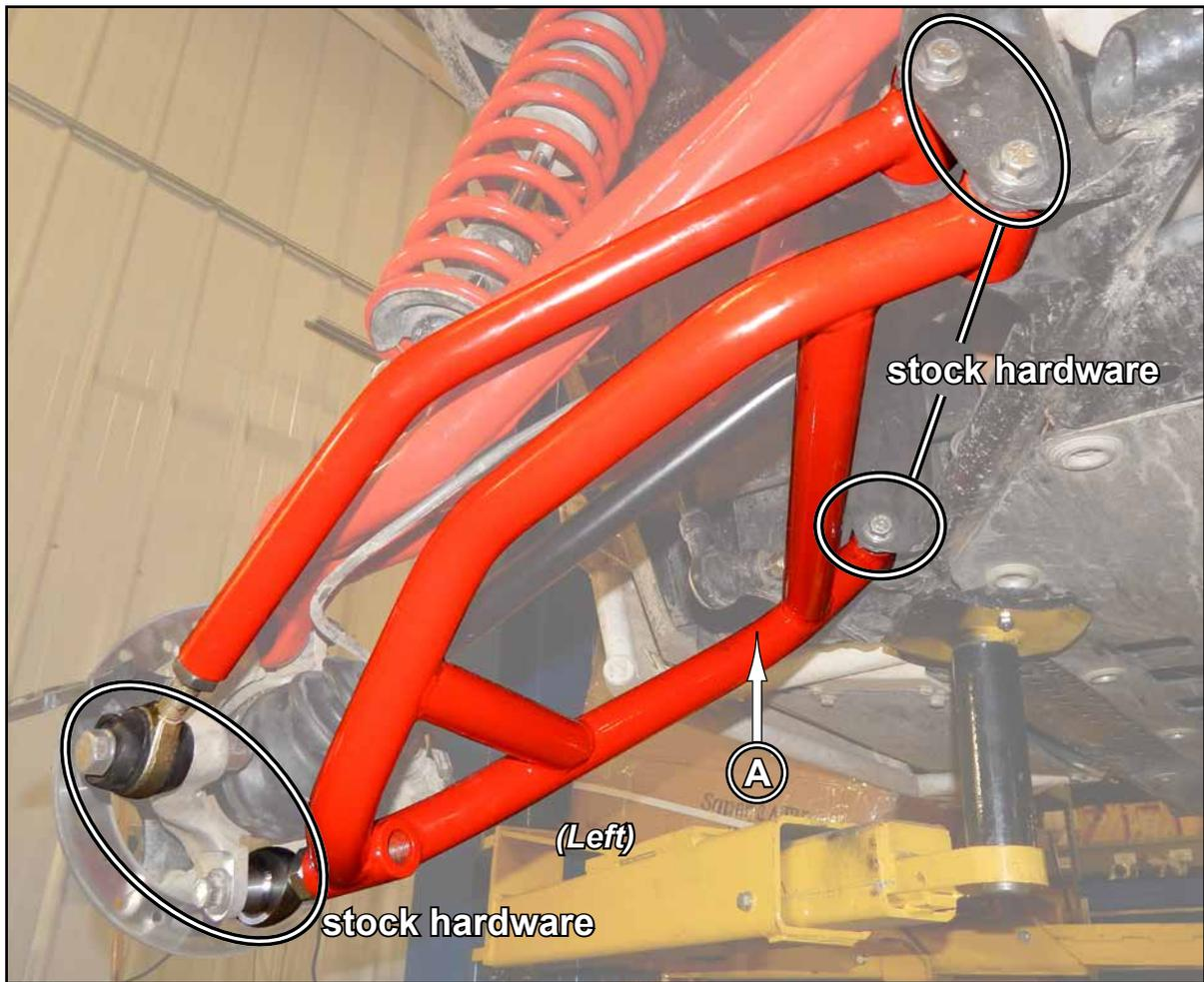
**SuperATV recommends using Loc-Tite on Nuts when installing A-Arms to Frame.**
