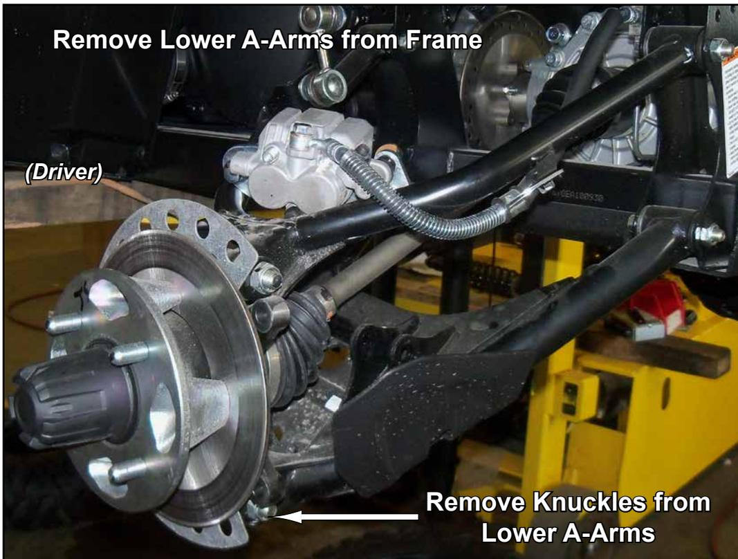
*SuperATV recommends using thread locker on nuts when securing components.*
