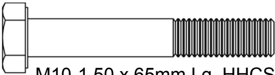
M10-1.50 x 65mm Lg. HHCS (H)
