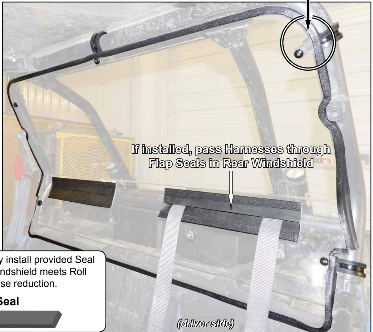
**Optional:** user may install provided Seal to places where Windshield meets Roll Cage for added noise reduction.
