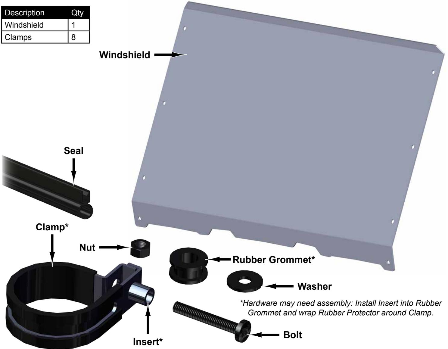
*\*Hardware may need assembly: Install Insert into Rubber Grommet and wrap Rubber Protector around Clamp.*
