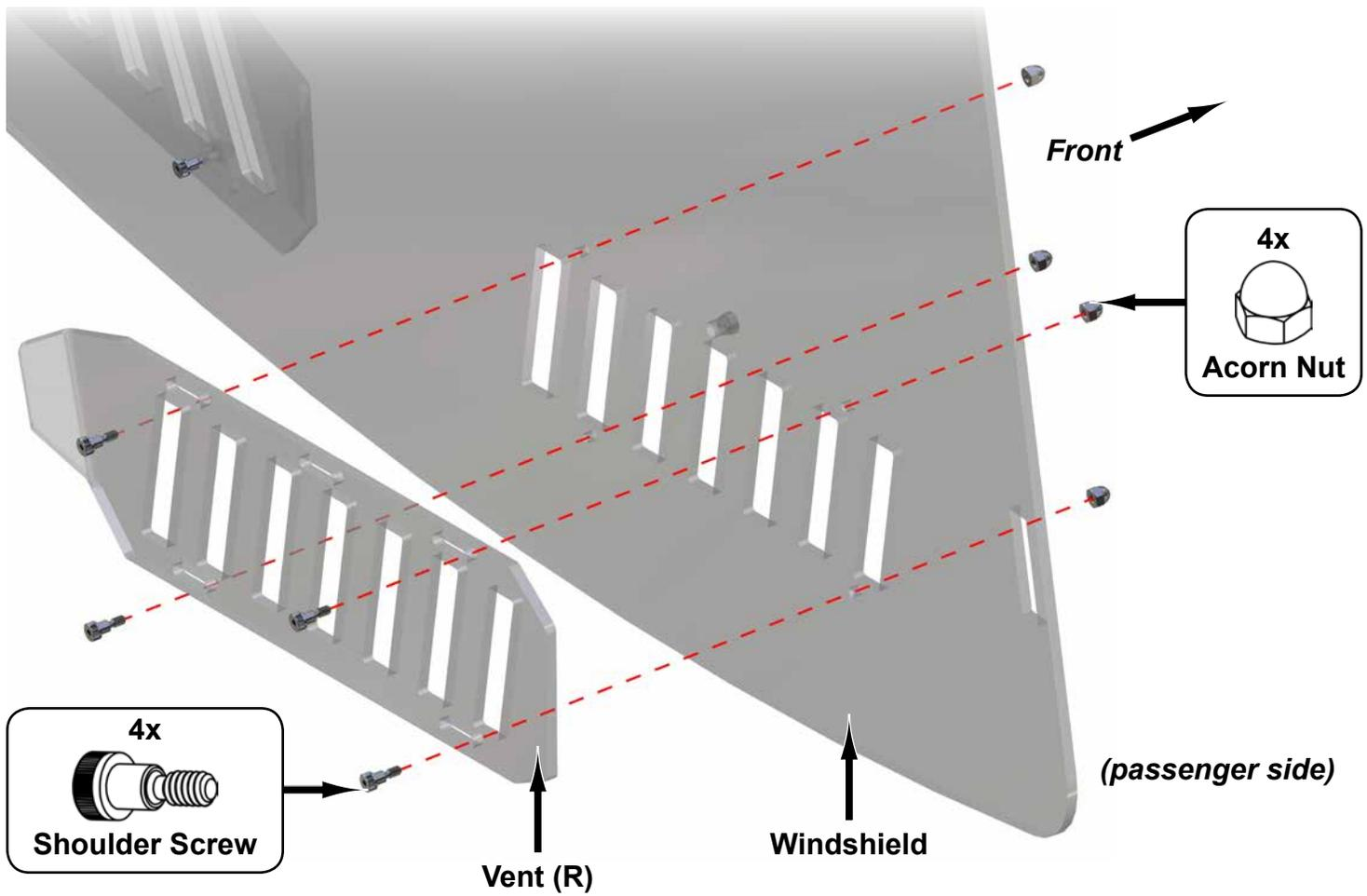
**Assemble Vents (R)(L) to Windshield with hardware shown.**
