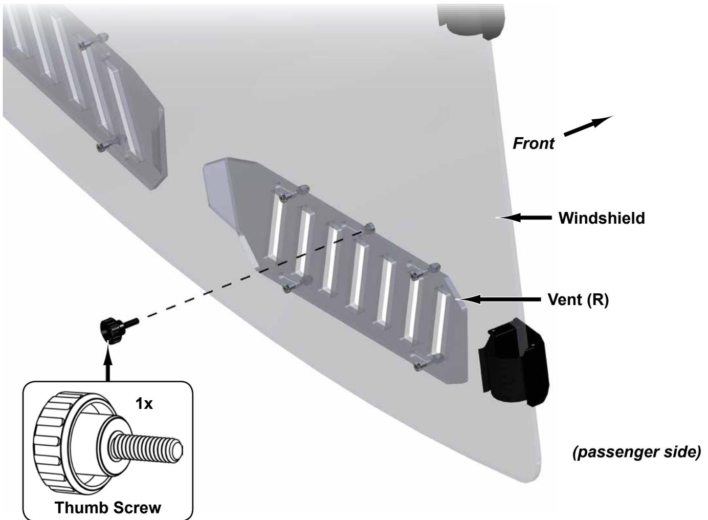
install Thumb Screw through each Vent and into factory installed Captive Nut.
