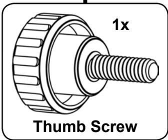
install Thumb Screw though each Vent and into factory installed Captive Nut.
