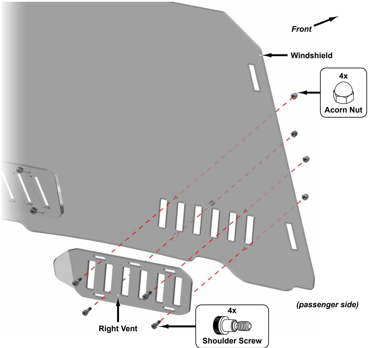
**Assemble Vents to Windshield with hardware shown.**
