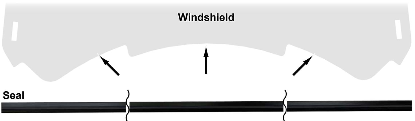
**Cut and install Seal to Windshield in (3) places shown.**
