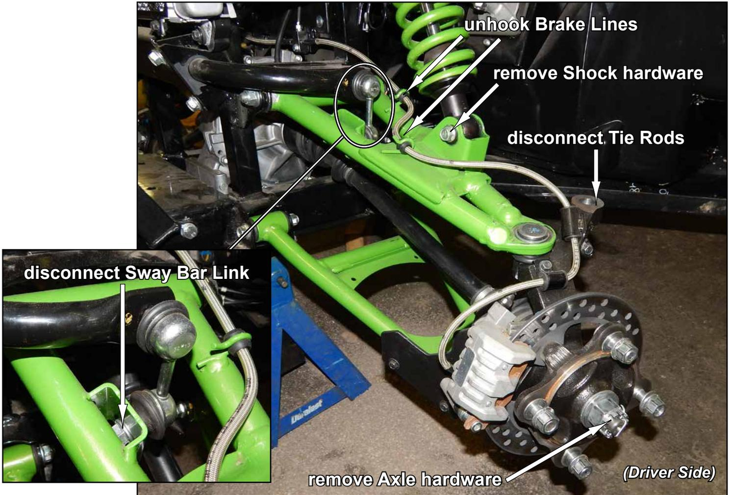
**Steering Stops installation:** *Note: Driver Side installation shown.*
